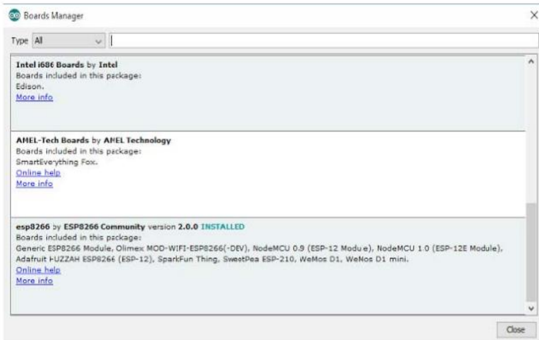
Figure 9: ESP 8266 board installation in Arduino
